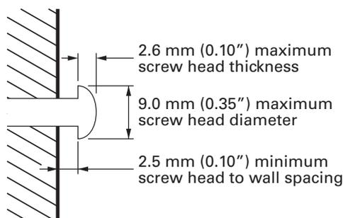
**Note:** If possible, mount the modem to concrete, masonry, a wooden stud, or some other solid wall material. Use anchor bolts if necessary (for example, if you mount the unit on drywall).
